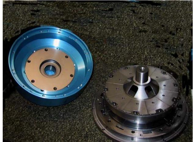
**Figure 4.** TIVM prototype assembled housings and expander rotor.
