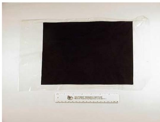
**Figure 2.** An 800-cm<sup>2</sup> active area MEA fabricated at SwRI.
