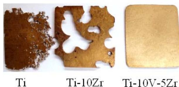
**Figure 1.** Nitrided model Ti-alloy coupons after 20 h immersion in 5% HF, illustrating that alloy composition can significantly influence the corrosion resistance of the resultant TiN-based surface layer.
