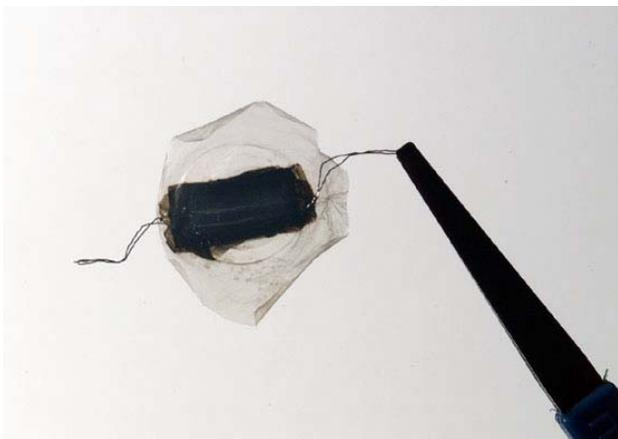
**Figure 3.** Membrane electrode assembly.
