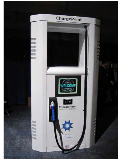
Above units use the JEVS105-1993 (JARI) DC coupler
