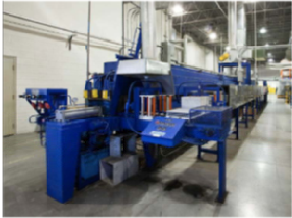
Figure 14: High temperature firing equipment for Versa Power's solid oxide fuel cells (ref. 26).
