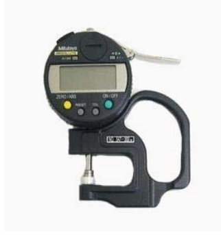
Figure 1.3. Mitutoyo Gauge for measuring thickness of membranes, CCMs, MEAs, and GDLs
