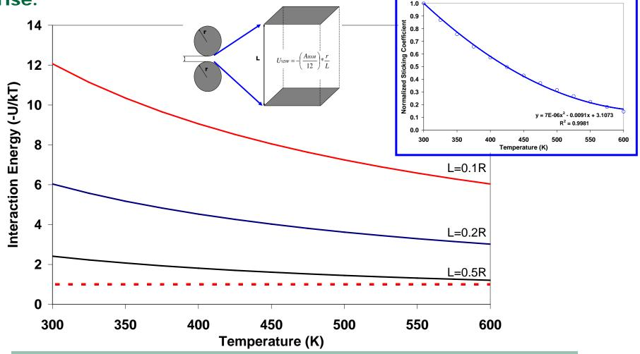
Reductions in thermophoretic and Van der Waals forces that occur simultaneously due to rising temperatures appear to contribute to the tendency for coolers to achieve a "stable" fouling state.
