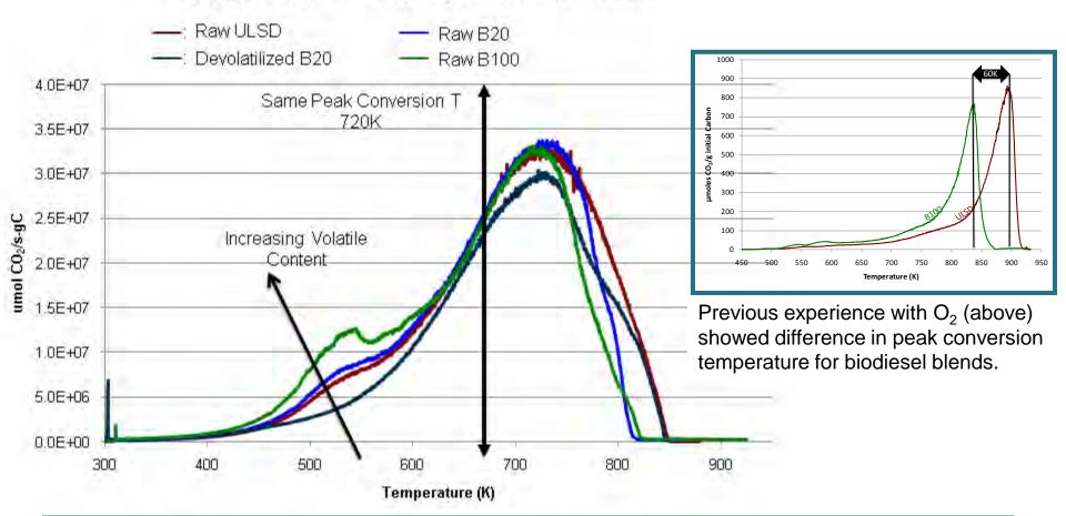
The collapse of fuel-related differences for oxidation by NO<sub>2</sub> (without normalization to surface area) implies a mechanistic difference for this oxidation pathway.
