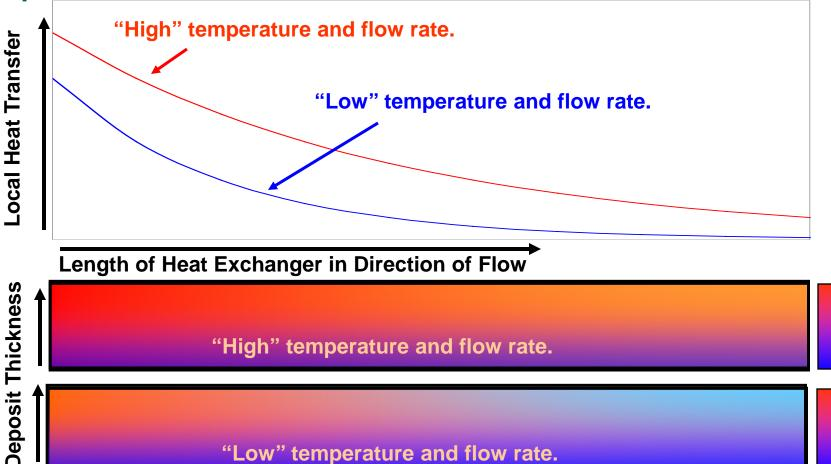
Use of a "large" heat exchanger at "low" heat transfer conditions can result in deposit layer temperatures conducive to HC deposition.
