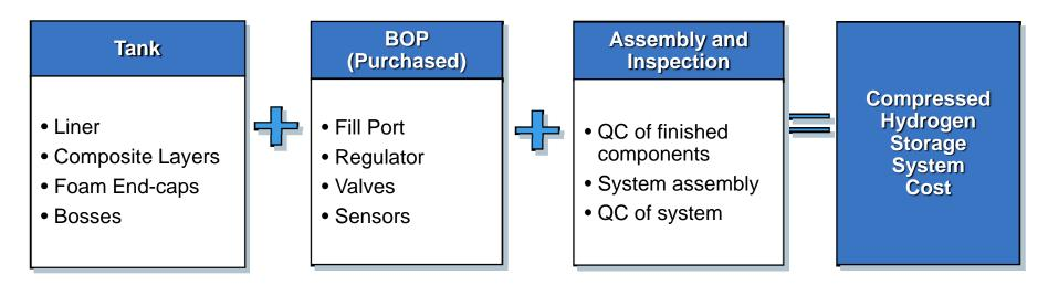
We modeled material and manufacturing process costs for the compressed tanks, while assuming that the BOP is purchased.
