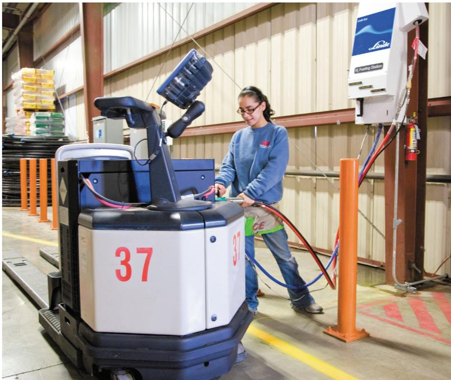
Operator makes hydrogen dispenser connections to a Class 3 material handling vehicle.
