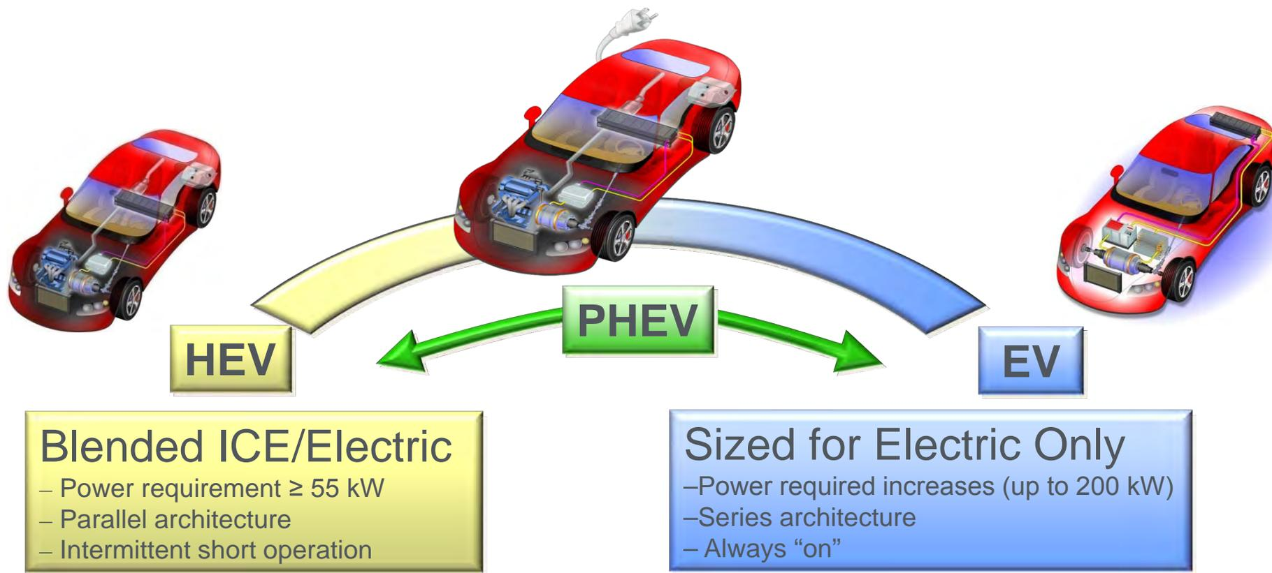
PHEV Position in Spectrum Depends on Design
