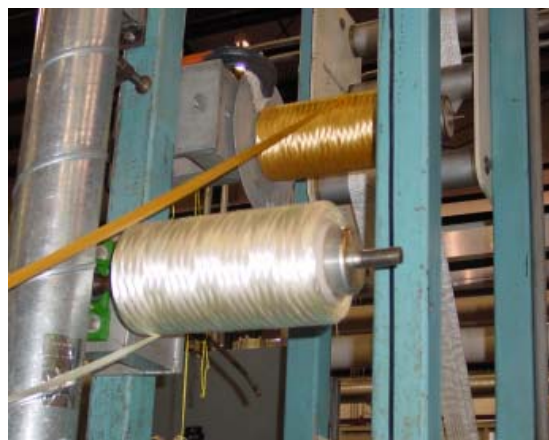
Figure 1: Typical Carbon Fiber Precursor (Front –Bottom) Chemically Pre-Treated Textile Based Carbon Fiber Precursor (Back – Top)
