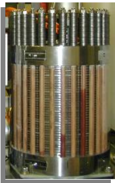
Figure 1: Giner Electrochemical Systems' 1,200 psig Electrolyzer
