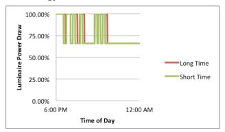
**Figure 16.** Sample data from an aboveground parking structure supporting an educational campus from 6:00 pm to midnight on a weekday. In the "long time" setting, the luminaire waits for 20 minutes after last activity is detected to go to the low setting. In the "short time" setting, the luminaire waits only for 10 minutes after last activity to go the low setting. The shorter the time delay, the greater the energy savings.
