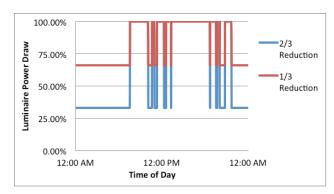
**Figure 15.** Sample data from an aboveground parking structure supporting an educational campus during the weekday. The figure depicts the usage when the low setting (when no activity is detected) is two-thirds and one-third full power. When the low setting is two-thirds reduction from full power, more energy is saved.
