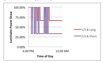
**Figure 17.** Sample data from an aboveground parking structure supporting an educational campus from 6:00 pm to midnight on a weekday. This graph compares little power reduction and a long time delay to a significant power reduction and a short time delay. Combining the short time delay with the greatest reduction in output permissible can optimize energy savings.
