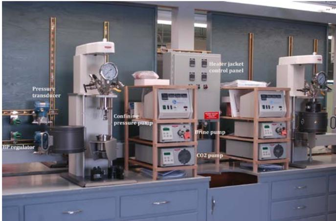
Example of flow-through system configuration
