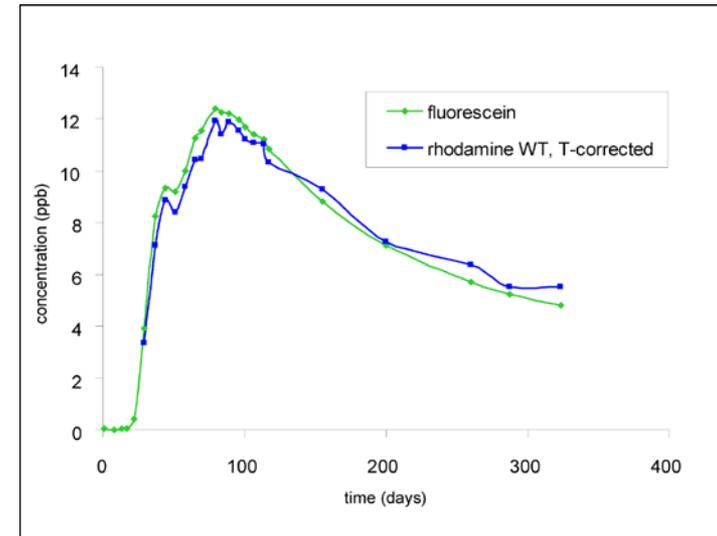
Tracer return curves from a test at Steamboat Springs involving the use of a thermally stable tracer in combination with a thermally reactive tracer.
