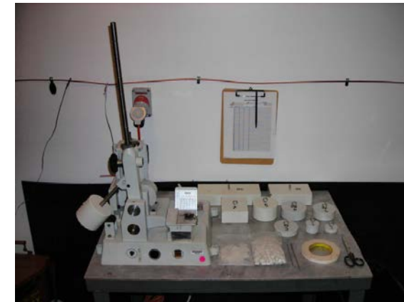
BAM Friction Apparatus
