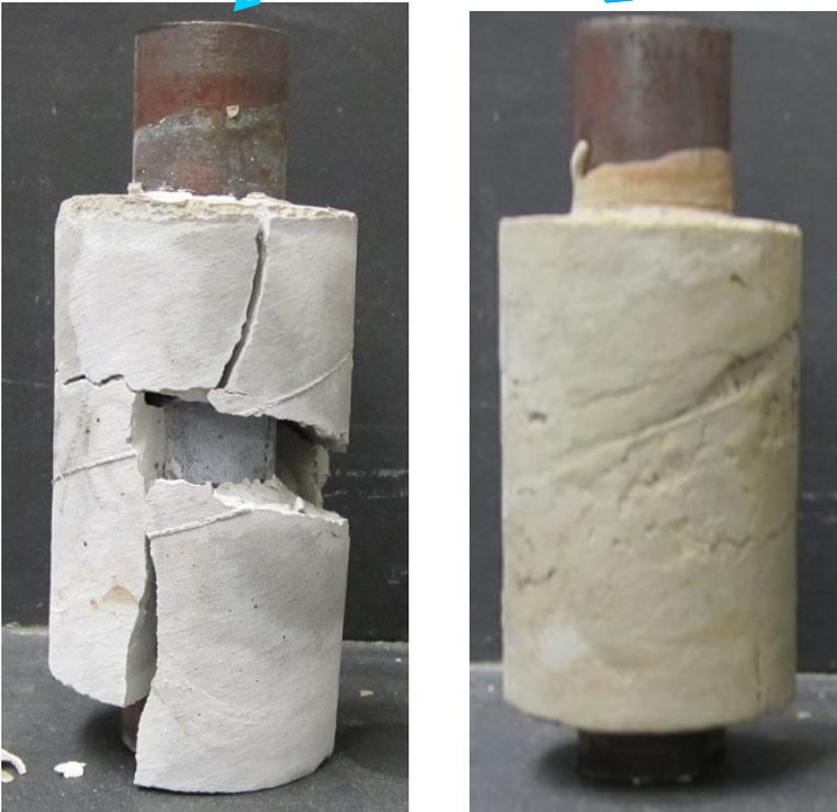
Shear bonding strength at interfaces between cement and casing before and after 5 cycle testing
