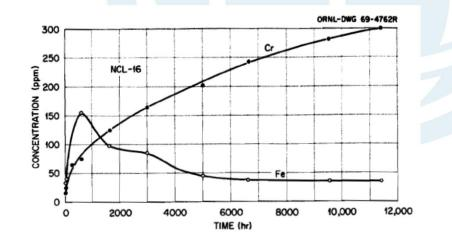
Reduction of  $FeF_2$  impurities causes Cr to be move from metal to salt. (ORNL-TM-4188)
