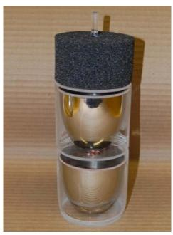
Corrosion samples will hang from quartz lids with Ni wire
