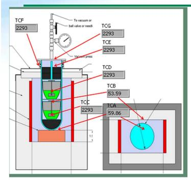
• Thermal profiling ensures uniform heating and adequate temperature control
