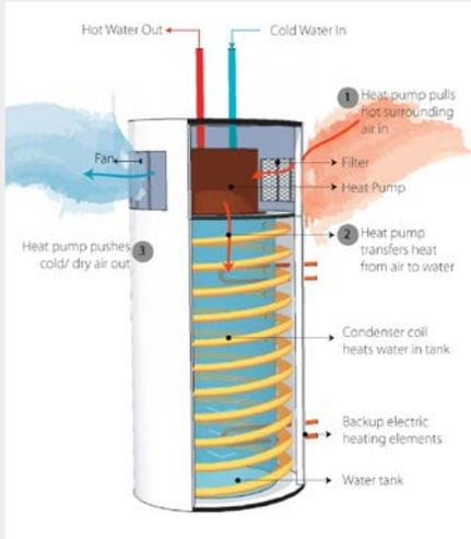
The most common arrangement of current HPWHs is an integrated water heater with a wraparound condenser and two backup electric elements. The figure above describes the typical components and operation of modern HPWHs in the U.S. market. Among the systems evaluated in this study, the only model to deviate from this configuration is the Stiebel Eltron unit, which has only one smaller (1.7 kW) upper element and always operates in hybrid mode.
