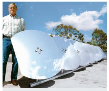
Self-powered, factory-assembled heliostats use closed-loop control to lower the cost of a solar collector field. Tower-mounted cameras sense reflections from small "solar proxies" mounted on each mirror; these reflections are then used to determine the real-time aiming point. *Photo from Thermata*
