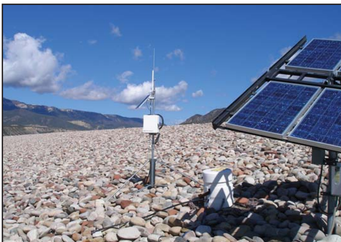
This SOARS monitoring station at the Rifle Disposal Site is powered by solar energy.
