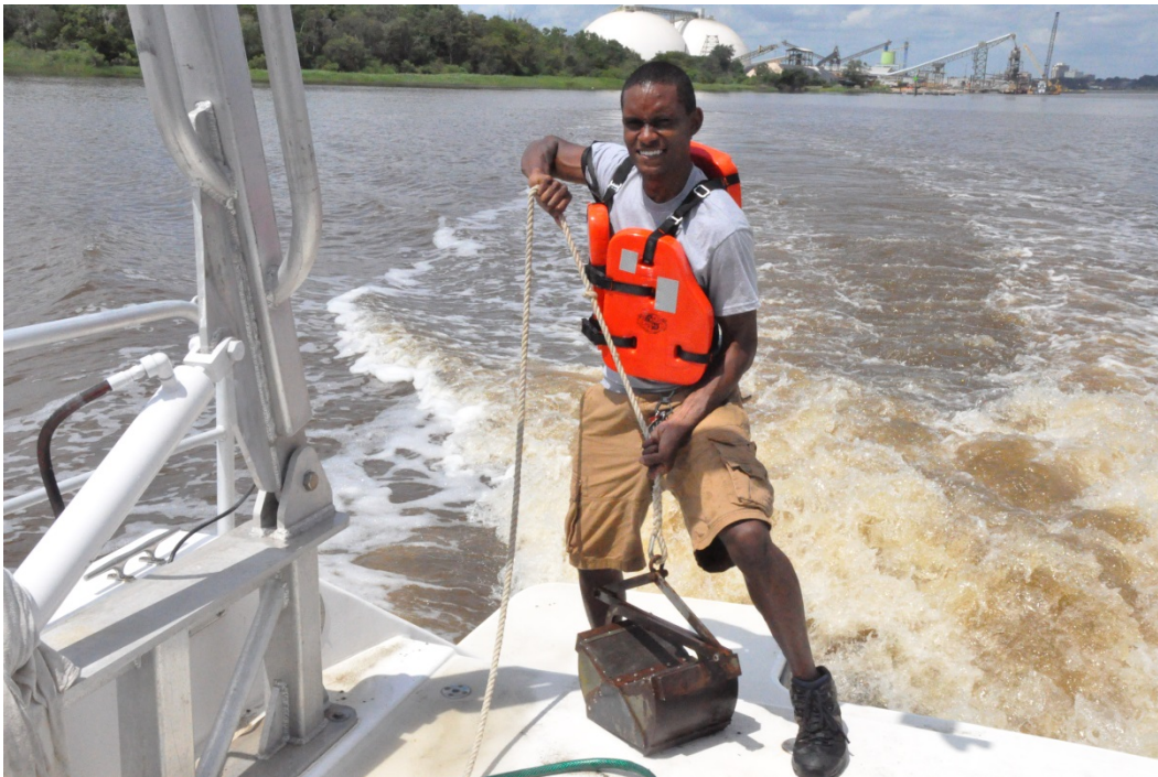
Mentors for Environmental Scholars intern collecting sediment samples for contaminant analysis from the Savannah River using a grab sampler.
