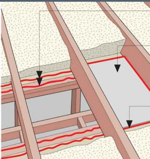
The *Guide to Attic Air Sealing* includes detailed drawings and step-by-step instructions for air sealing common air leaks into attics.
