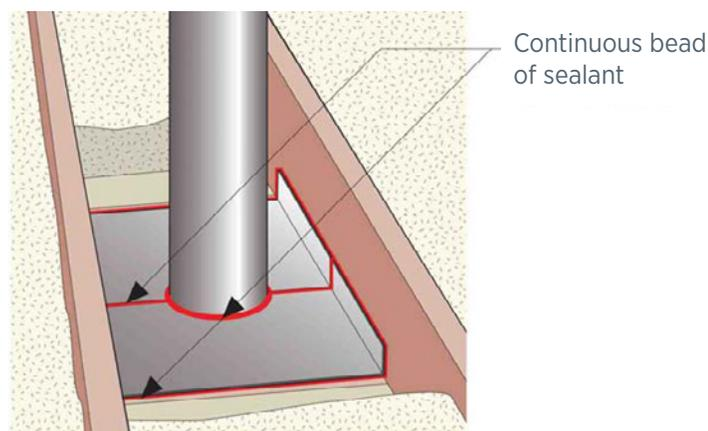
Drawings and instructions in the guide show contractors the proper way to air seal around typical breaks in the ceiling. Here, sheet metal and fire-rated caulk provide air sealing around a flue pipe.
