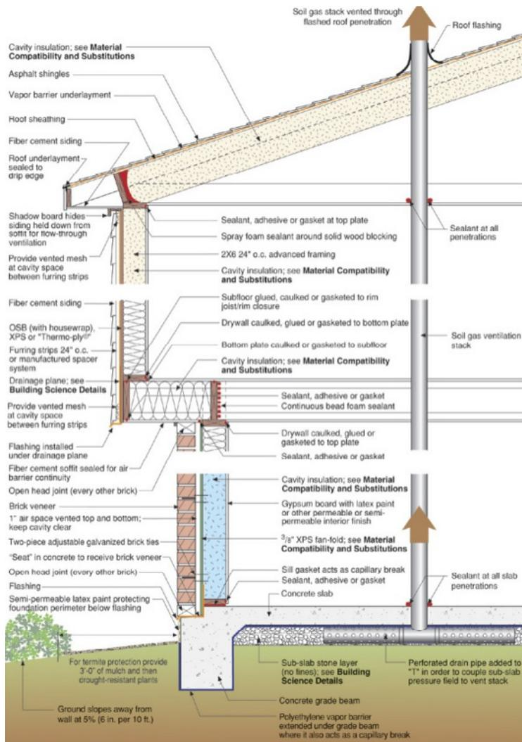
Building Science Corporation developed detailed schematics for enclosures that work in each climate zone.
