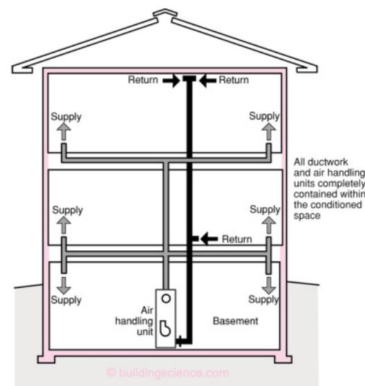
Ducts can be located in conditioned space in A) an insulated attic, B) a dropped ceiling chase, or C) between floors.
