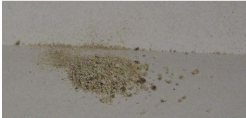
Dried mineral precipitate from inlet strainer
