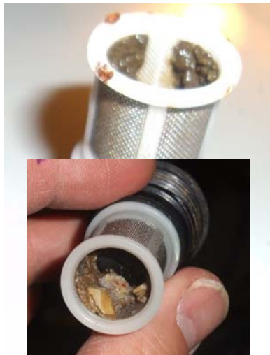
Same operational problems with inlet strainer clogging, plus more!
