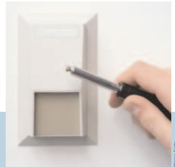
Temperature sensors must be calibrated against known standards to ensure that monitoring results and actual comfort conditions match.
