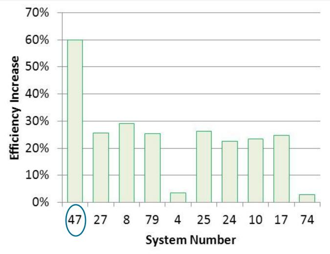
High SEER & AFUE – but very small return air grille (14 x 24) with 14" duct – improved from 252 to 371 CFM/ton with 2<sup>nd</sup> return
