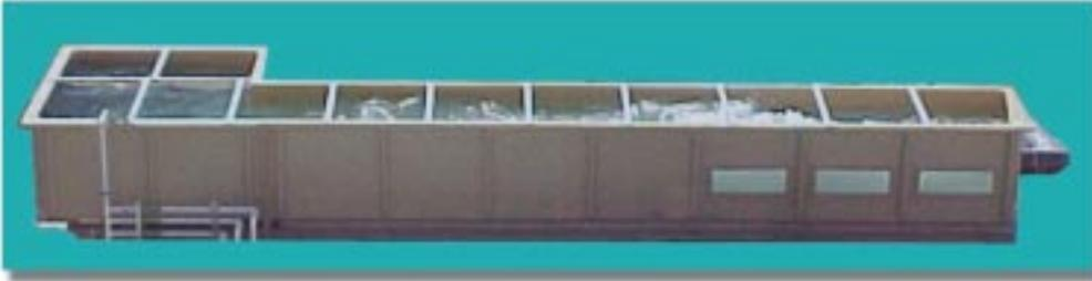
*High-velocity test flume showing flow from right to left. The flume measured 9 m long x 1.2 m wide x 1.2 m deep. An electric pump capable of producing exit velocities in excess of 20 m/s was used to produce a consistent shear environment. Viewing windows at the sides and bottom were inserted to facilitate video recording.*
