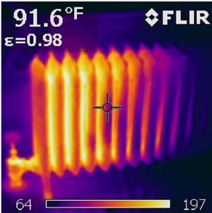
Properly functioning radiator vents allow air to escape and steam to fill the radiator.
