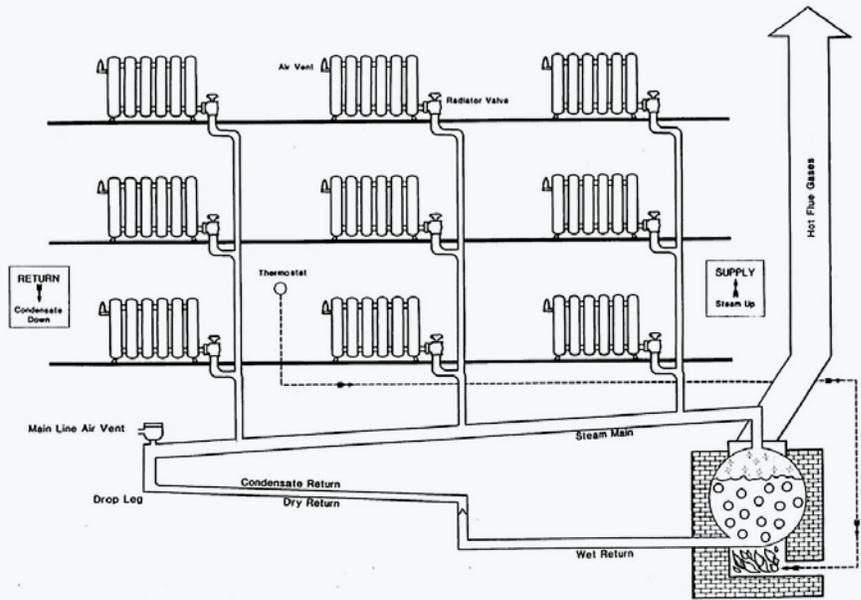
In a one-pipe steam system, there should be a main line vent at the end of each steam main, about 15 in. before the piping drops down into a return. Each radiator should have a properly sized and functional air vent.
