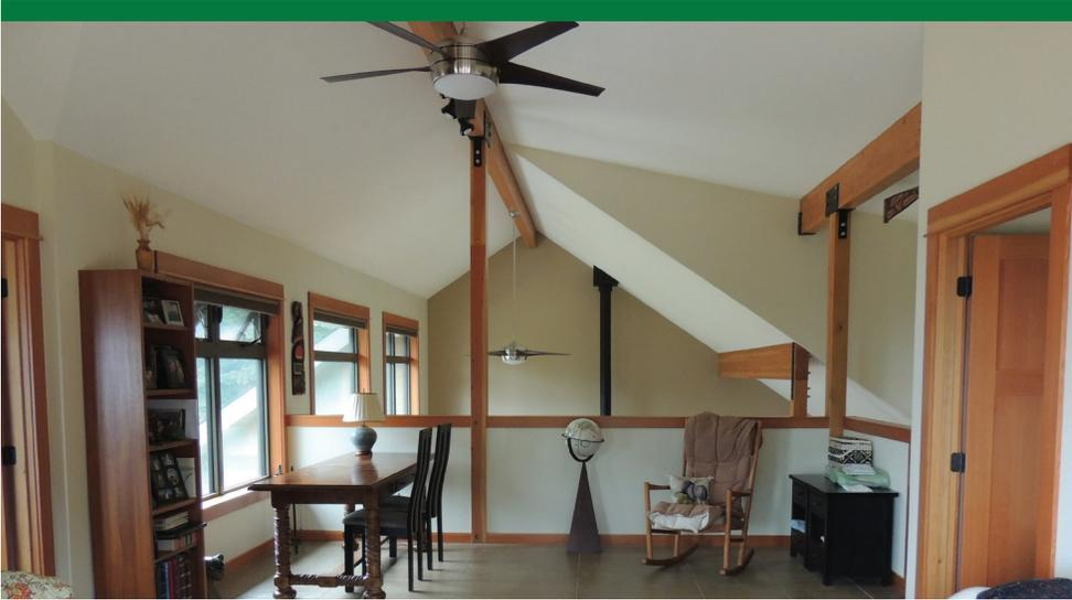
Large south-facing windows allow any available sunlight to warm up the concrete flooring on the first and second floors. These thermal mass floors absorb solar energy during the day and radiate the heat into the space throughout the night. Deep overhangs block out high summer sun and an innovative ventilation system that uses multiple timed exhaust fans to pull air into and out of the house can remove unwanted heat during the early morning hours in the summer.
