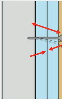
Vertical movement resistance provided by friction between layers.
