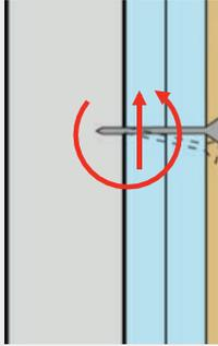
Rotational resistance provided by tension in fastener and compression of the insulation.
