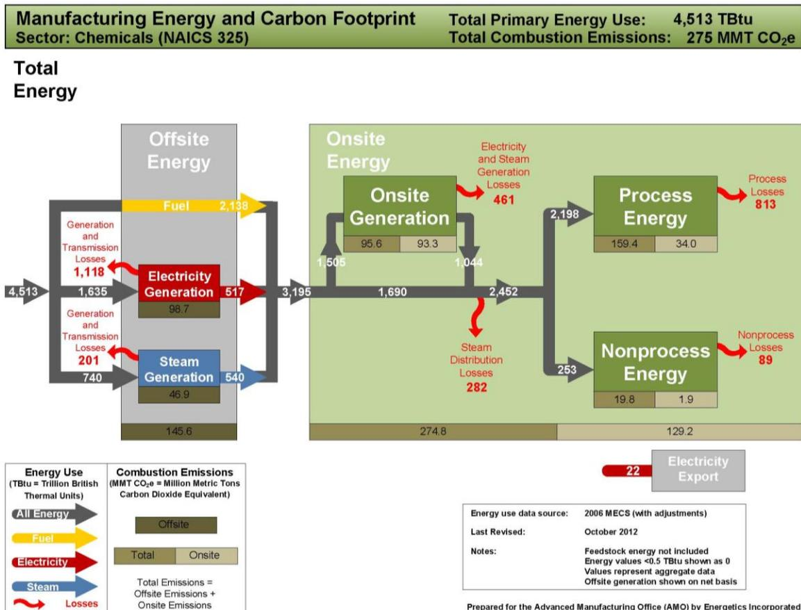
Figure 2: Total primary energy use and GHG combustion emissions for the chemicals sector
