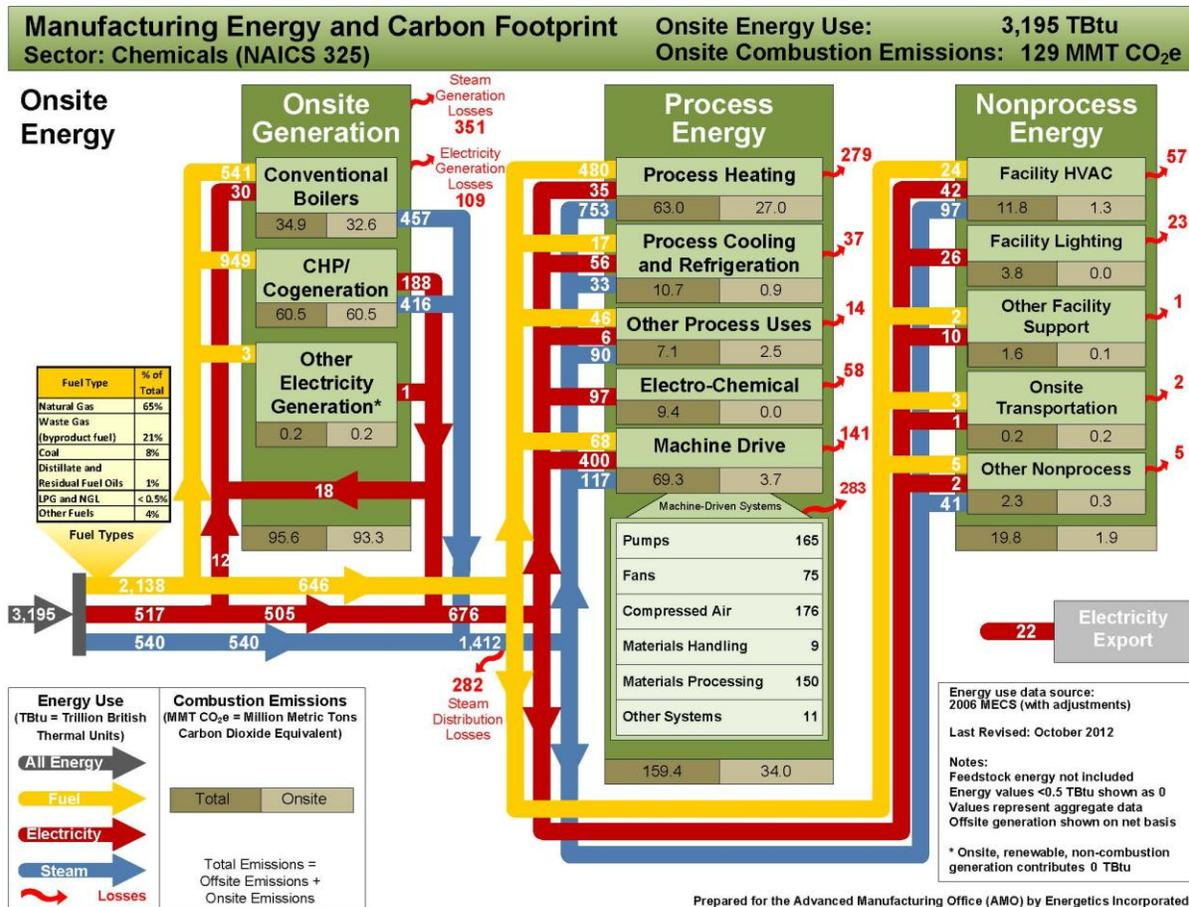
Figure 3: Onsite energy and carbon emissions for the chemicals sector
