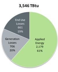
Fig. 2.4-12. Primary energy by loss and applied energy in the petroleum refining sector
