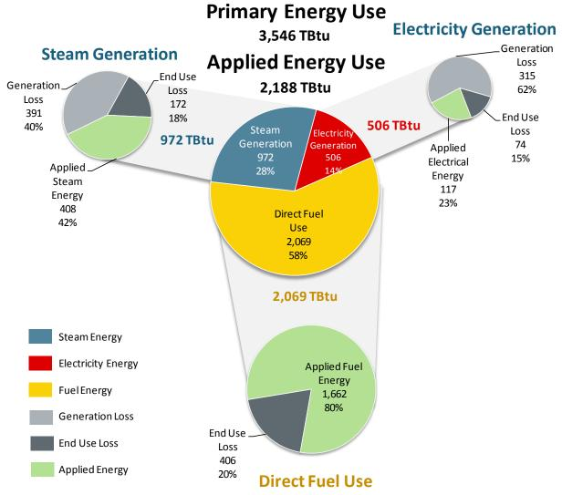
Fig. 2.4-11. Primary energy and applied energy by energy type in the petroleum refining sector
