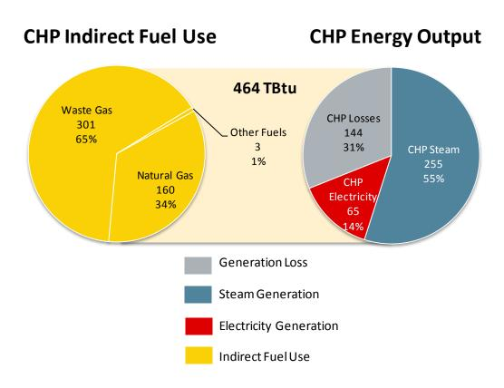
Fig. 2.4-8. CHP fuel consumption and energy output in the petroleum refining sector
