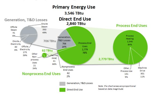
Fig. 2.4-10. Primary energy by *direct* end use in the petroleum refining sector
