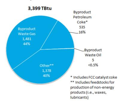
Fig. 2.4-1. Feedstock energy use in the petroleum refining sector
