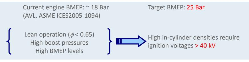
Though noble metal (Platinum & Iridium) electrodes are used, durability of spark plugs is still a concern
