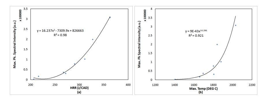
Potential use of flame emission to monitor Heat Release Rate & Peak cycle temperature in natural gas engines
