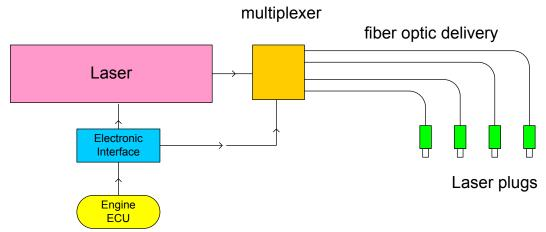
Pulsed output of a single laser multiplexed to different cylinders. Developed a prototype system
