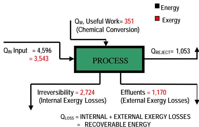
Figure 4b: Energy and Exergy Losses- Base Ammonia Process (Btu/lb of Ammonia)
