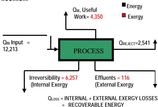
Figure 2A: Summary of Energy and Exergy Losses in Alternative Chlorine-Caustic Technology (Membrane Retrofit of Diaphragm Process Btu/lb of Cl<sub>2</sub>)
