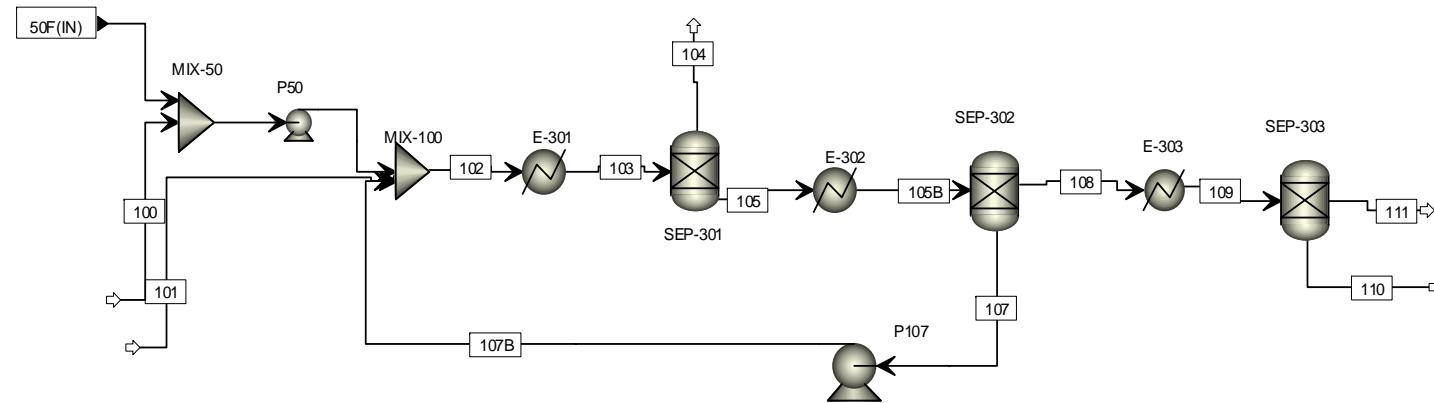
**Figure 5D – Base Terephthalic Acid Case – pt 1**
