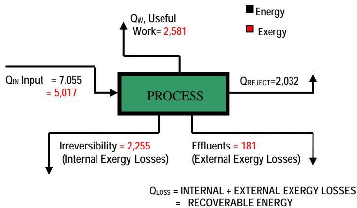
Figure 1A: Energy and Exergy Losses in Alternative Ethylene Process Technology
