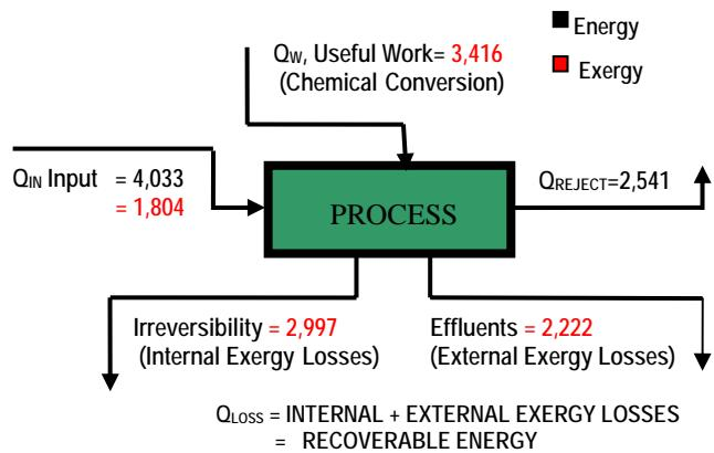
Figure 5A: Summary of Energy and Exergy Losses for Alternative Terephthalic/Isophthalic Process Technology (Btu/lb of PTA+IPA)
