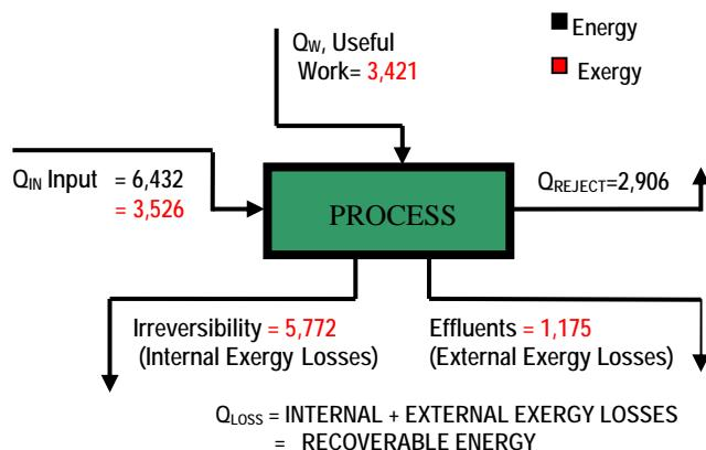
Figure 3B: Energy and Exergy Losses in NEW Base Ethylene Oxide Process (Btu/lb of EO)
