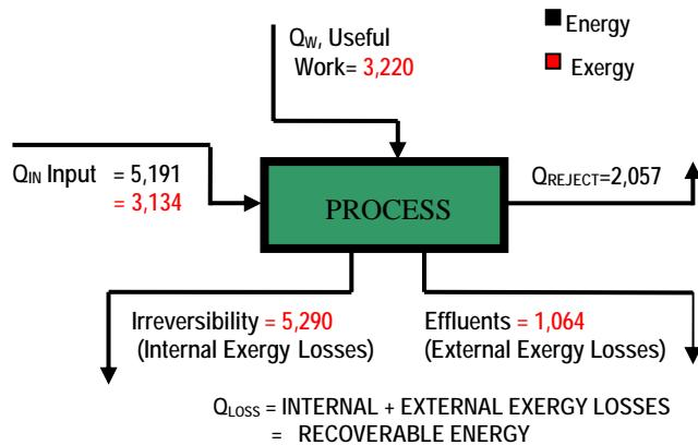
Figure 3A: Energy and Exergy Losses in Alternative Ethylene Oxide Process Technology utilizing Microchannel Reaction System (Btu/lb of EO)
