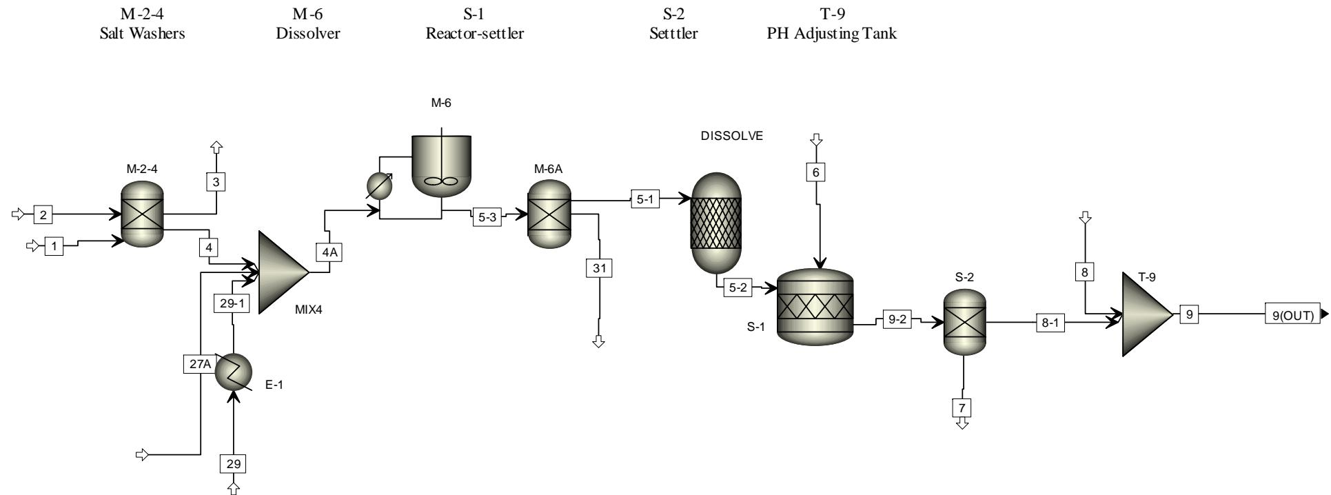
**Figure 2C – Alternative Chlorine – Caustic Soda – part 3**
