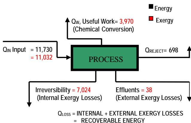
Figure 2B: Energy and Exergy Losses- Base Chlorine-Caustic Diaphragm Cell Process (Btu/lb of Cl<sub>2</sub>)
