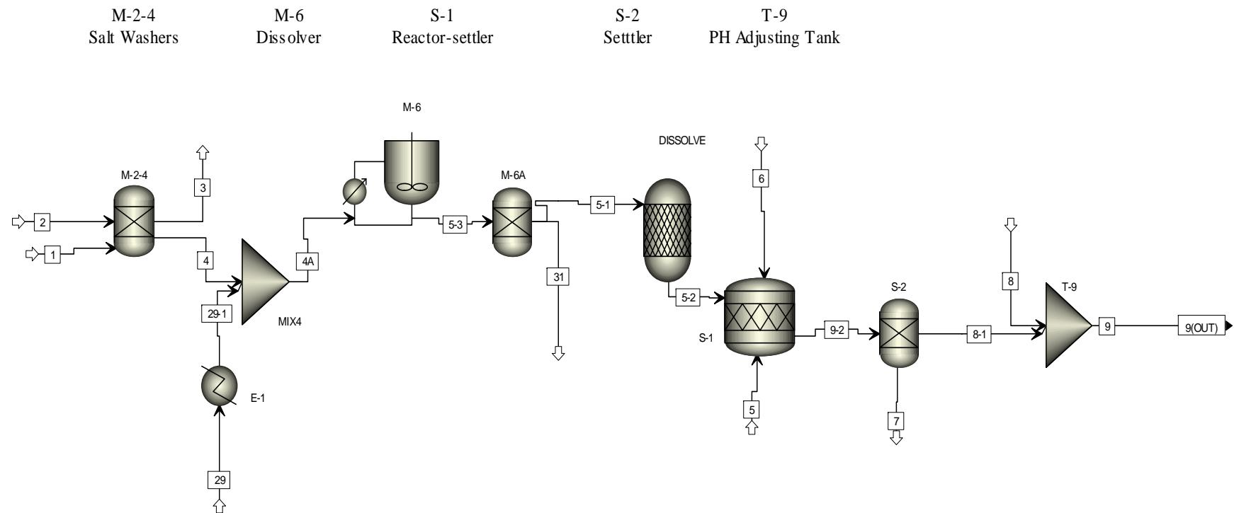
**Figure 2G – Base Case Chlorine – Caustic Soda – part 3**
