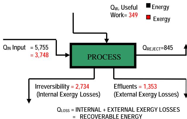
Figure 4A: Summary of Energy and Exergy Losses for Alternative Ammonia Process Technology with PSA Elimination of Recycle NH3 (Btu/lb of NH3)
