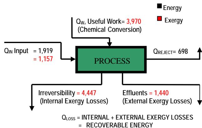
Figure 5b: Energy and Exergy Losses- Base PTA (Purified Terephthalic Acid Process (Btu/lb of PTA))
