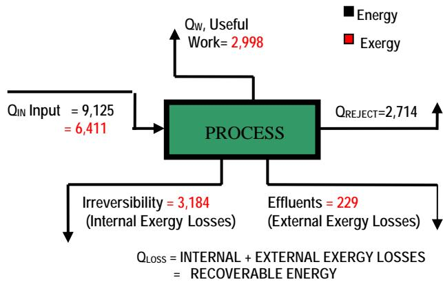
Figure 1B: Energy and Exergy Losses in Base Ethylene Process (Btu/lb of Ethylene)
