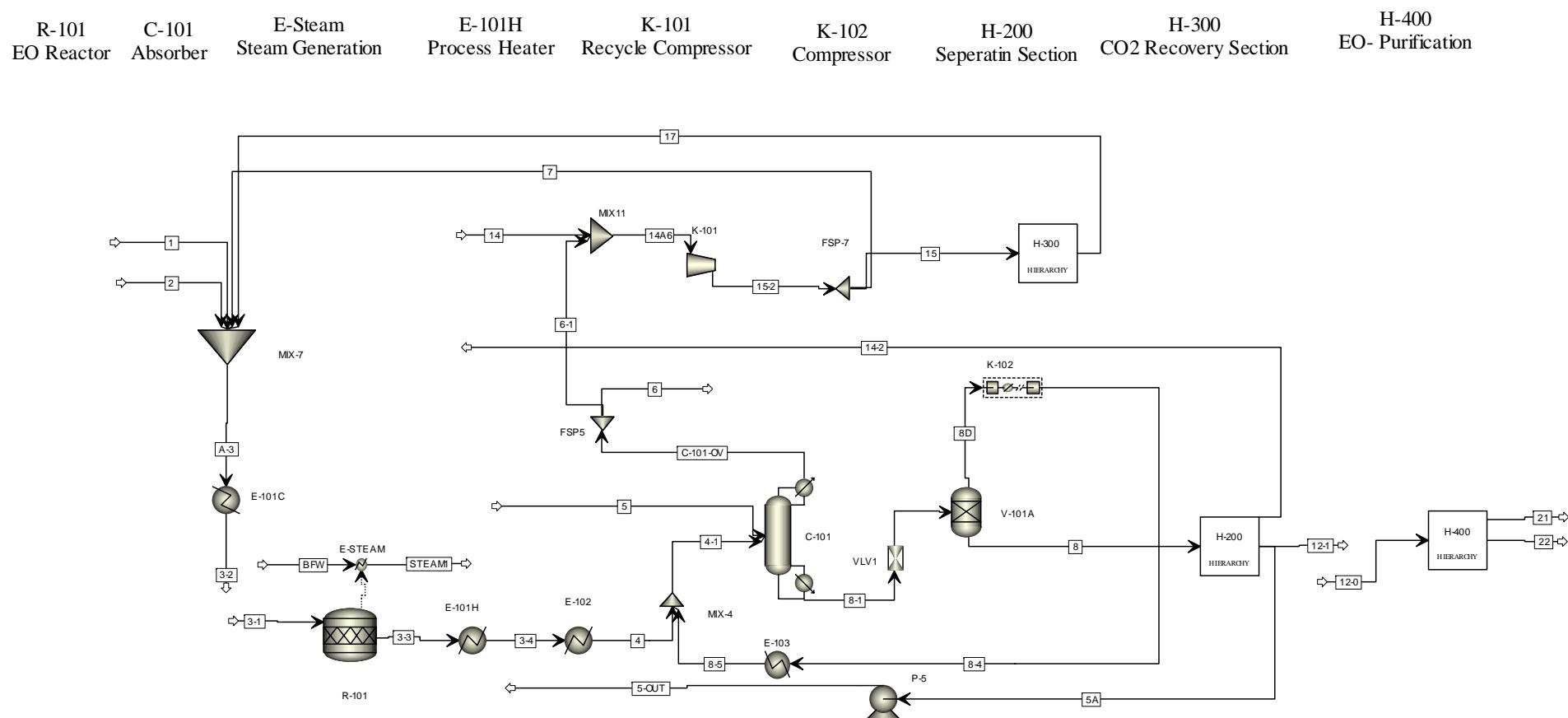
**Figure 3B – Alternative Ethylene Oxide Process – Pt 2**
