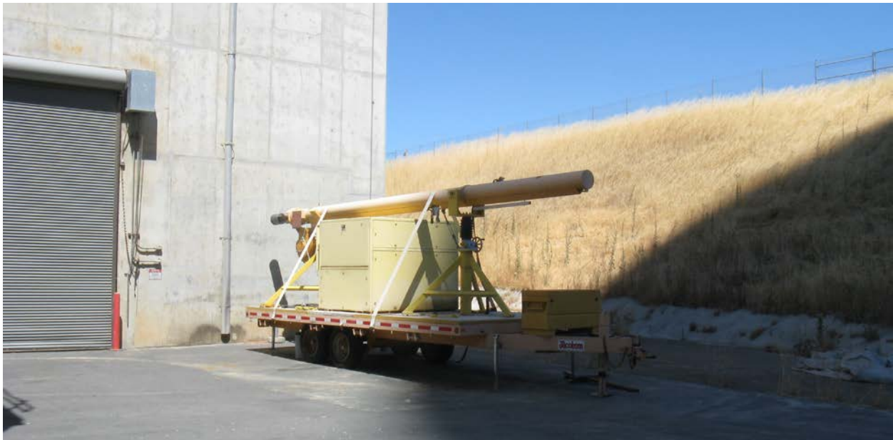
Figure 2-78. Hydraulic Ram Used to Emplace and Withdraw Canisters from Horizontal Storage Modules at Rancho Seco
