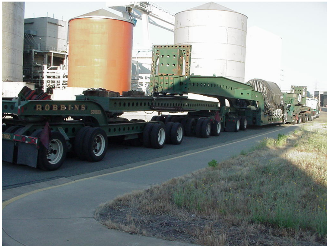
Figure 2-85. MP187 Cask Transported by Heavy Haul Truck
