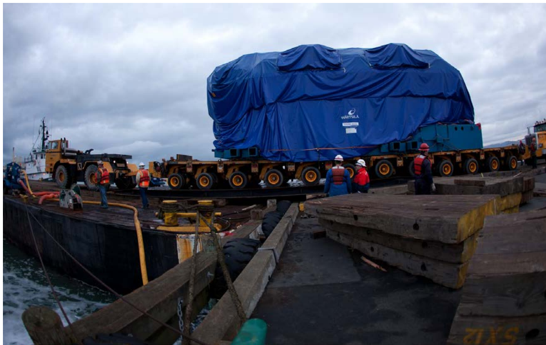
Figure 2-48. Wartsila Engine Being Loaded on a Barge
