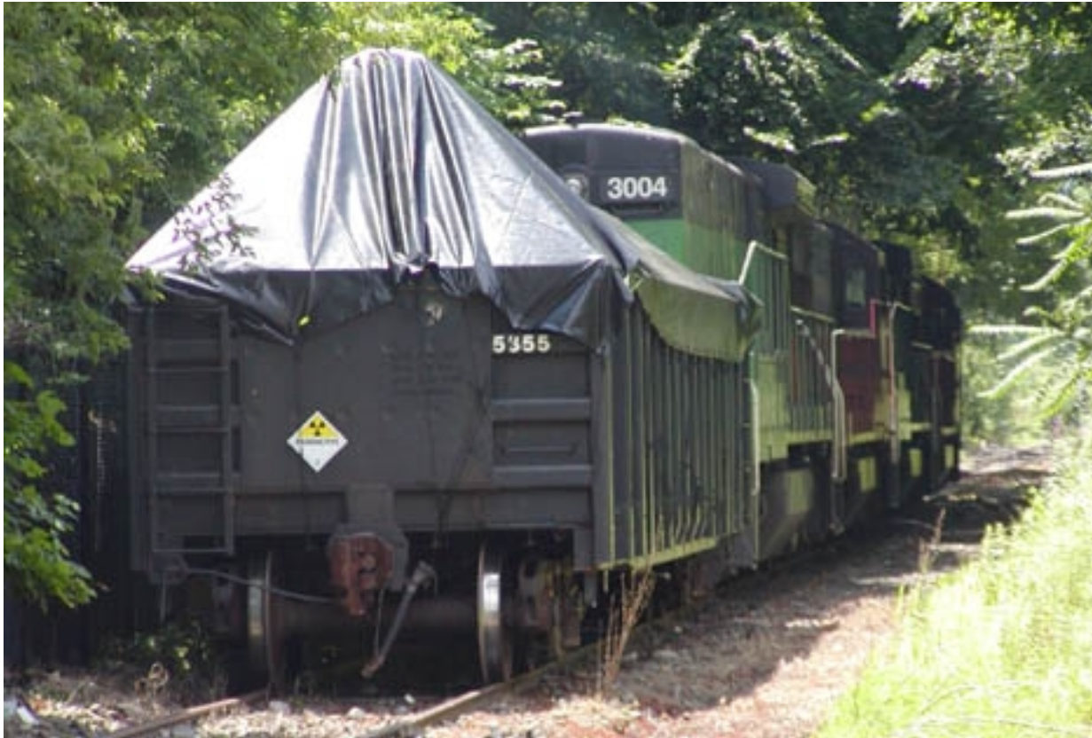
Figure 2-35. Connecticut Yankee Pressurizer at Portland Railhead
