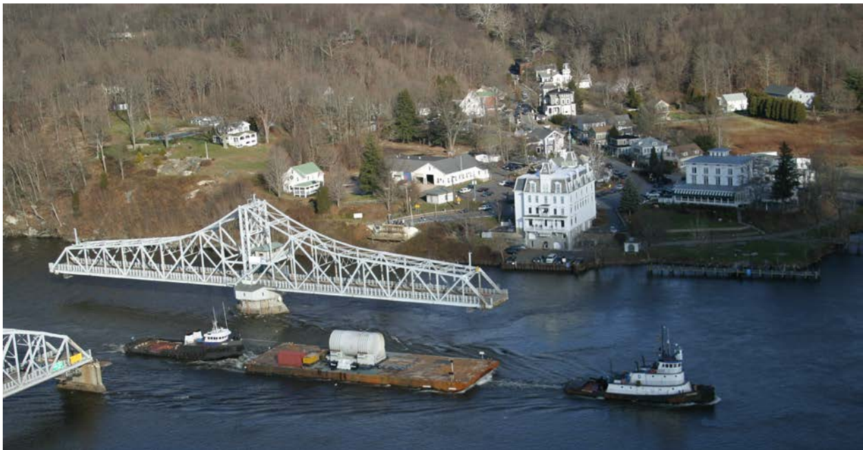
Figure 2-39. Connecticut Yankee Reactor Pressure Vessel Being Transported on Barge in the Connecticut River
