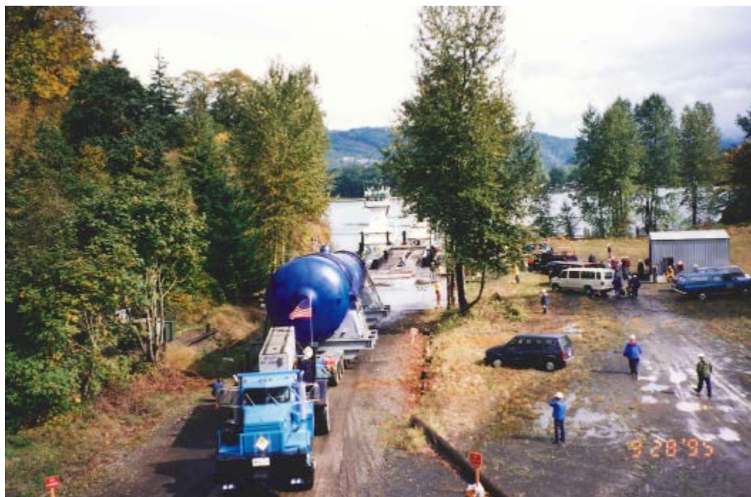
Figure 2-99. Trojan Steam Generator Being Loaded at Barge Slip
