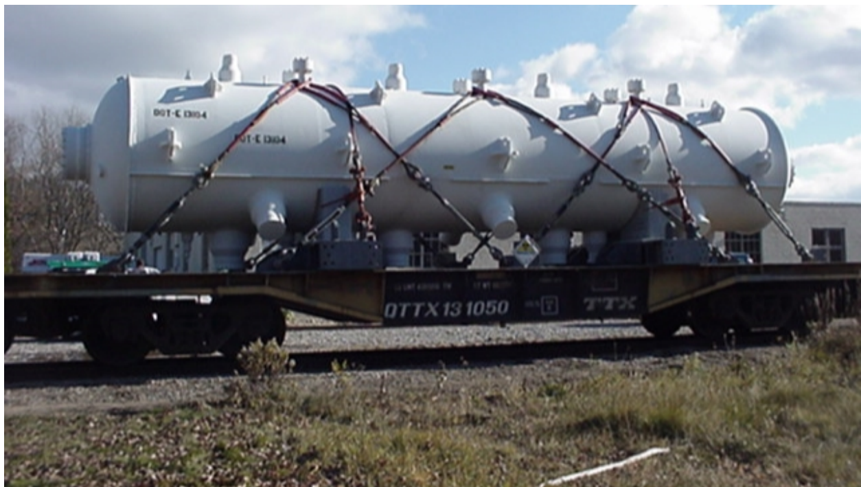
Figure 2-72. Big Rock Point Steam Drum on Railcar
