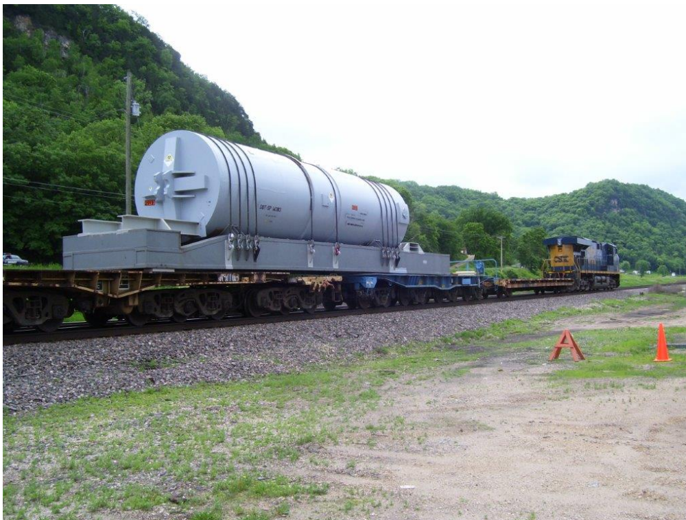
Figure 2-112. La Crosse Reactor Pressure Vessel on BNSF Railroad
