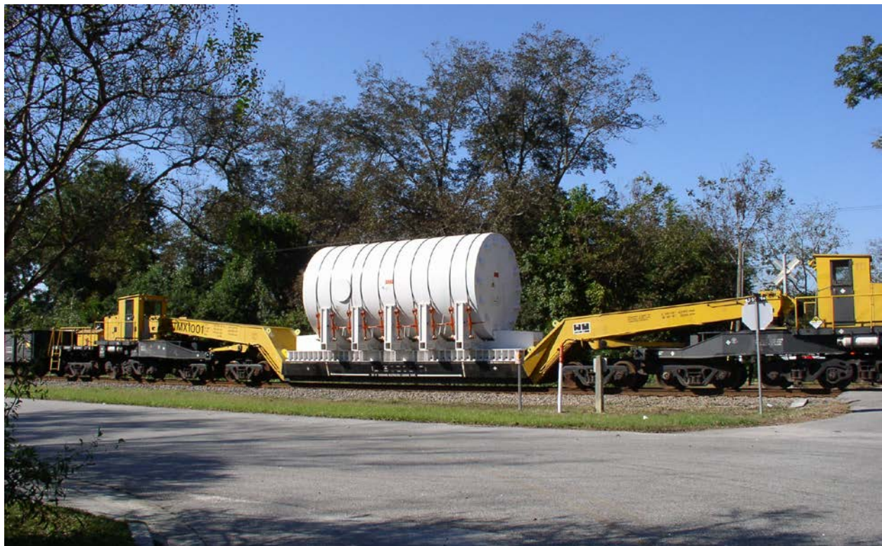
Figure 2-64. Big Rock Point Reactor Pressure Vessel on Railcar
