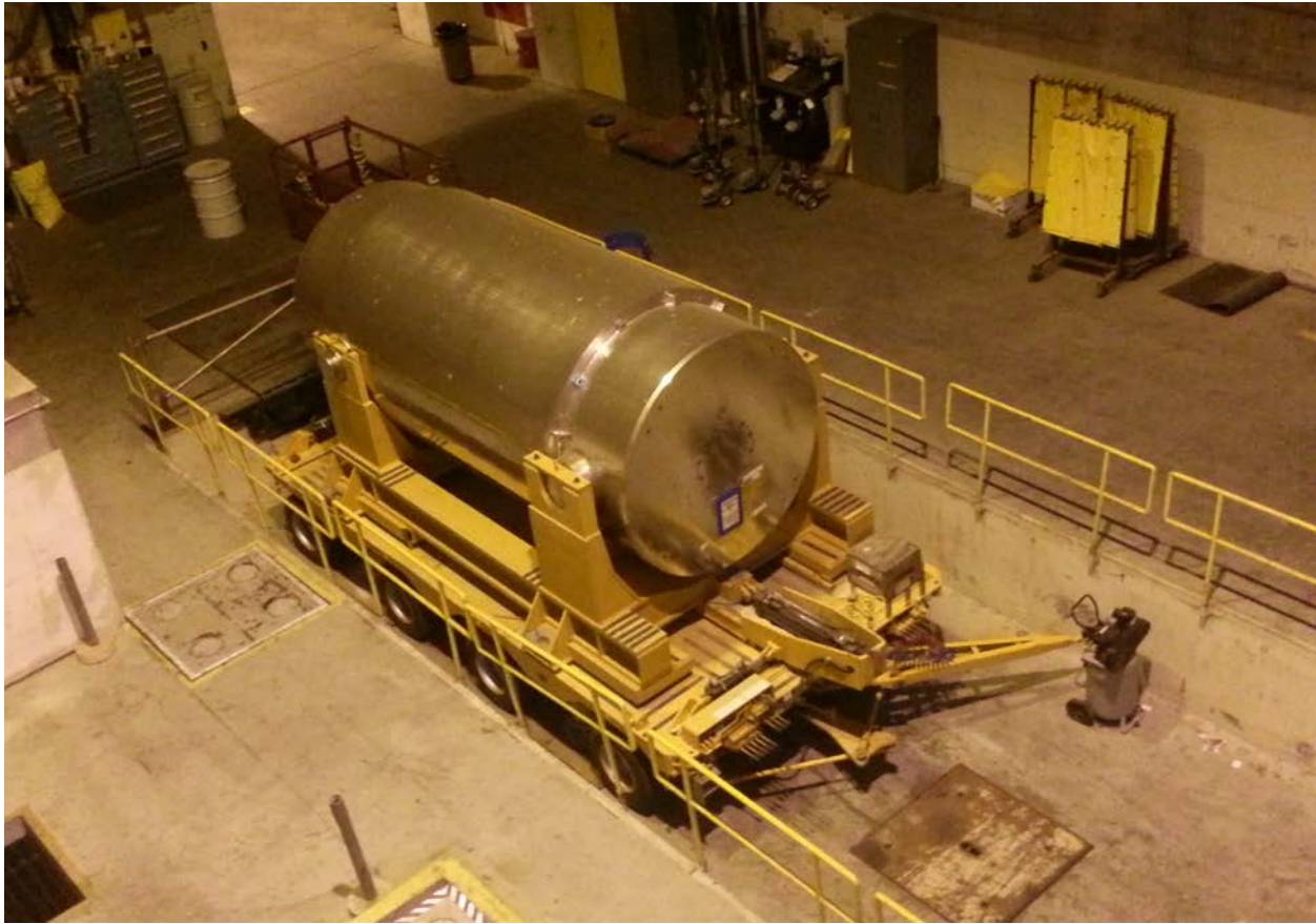
Figure 2-77. MP187 Transportation Cask at Rancho Seco
