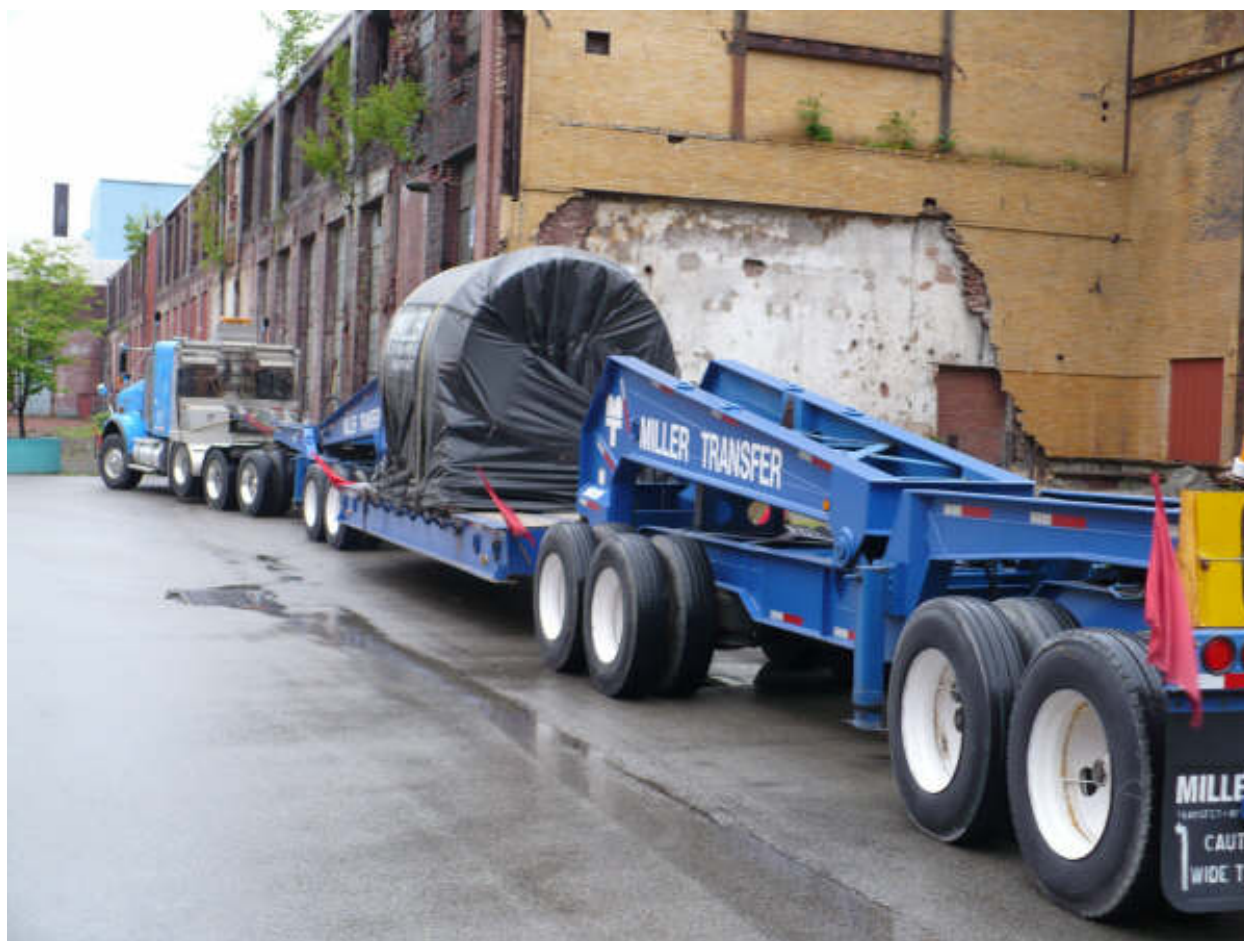
Figure 2-44. Empty HI-STAR HB Cask Transported by Heavy Haul Truck
