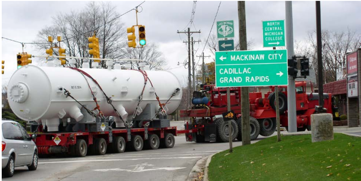
Figure 2-71. Big Rock Point Steam Drum on Heavy Haul Truck
