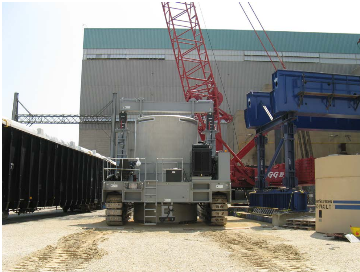
Figure 2-120. Transporter Used to Move Vertical Concrete Storage Casks
