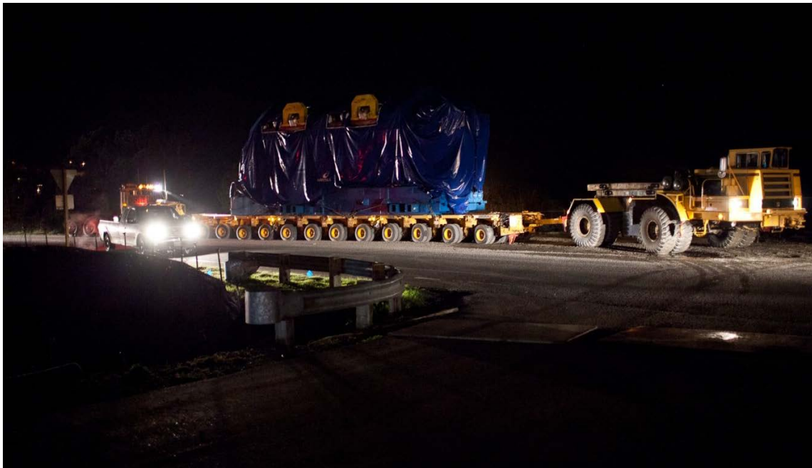
Figure 2-52. Wartsila Engine Being Transported by Heavy Haul Truck to Humboldt Bay Generating Station
