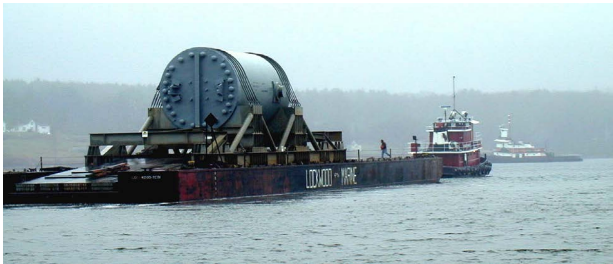
Figure 2-16. Maine Yankee Reactor Pressure Vessel Being Transported on Barge
