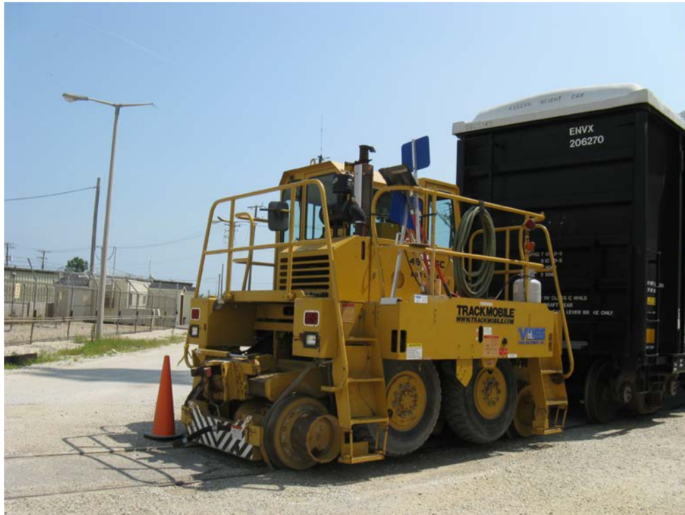
Figure 2-122. Trackmobile Used to Move Railcars On-site
