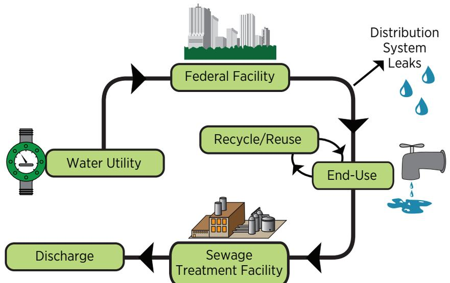
The water distribution cycle for Federal buildings starts at the water utility and ends when water is discharged back into the environment.
