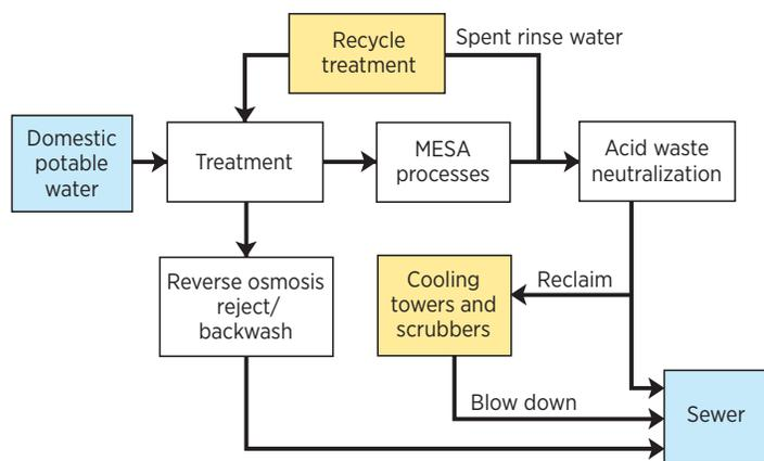
This simplified flow chart shows the general path of the recycled and reclaimed water in the MESA plant.
