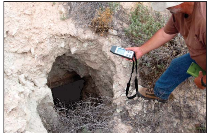
Field personnel collecting gamma exposure-rate measurements at a subsided mine portal in the Yellow Cat mining area of Grand County, Utah.
