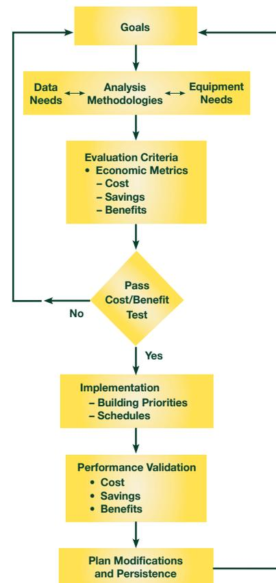
Figure 8.8.1. Development process for meter system planning
