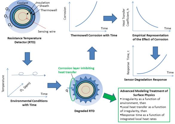
Process for "Re-Calibrating" Sensor
