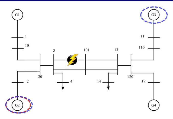
Increase tie line impedance increased by 10% and disable the PSS to reduce the damping
