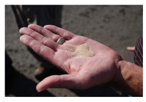
Fine-grained silica sand is mixed with chemicals and water before being pumped into rock formations to prevent the newly created artificial fractures from closing after hydraulic fracturing is completed. Photo: Bill Cunningham, U.S. Geological Survey
