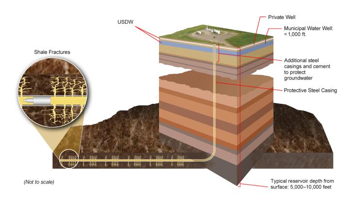
Producible portions of shale gas formations are located many thousands of feet below the surface, well below groundwater aquifers. Modern hydraulic fracturing technology involves sophisticated engineering processes designed to create distinct fracture networks in specific rock strata. Experts continually monitor all aspects of the process, which must comply with local, state and federal laws and regulations.
