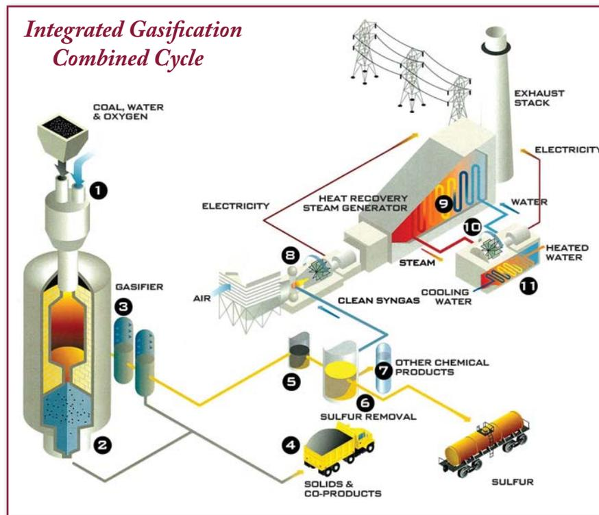
1. Coal, water, and oxygen are fed into a high-pressure gasifier, where the coal is partially combusted and converted into synthetic gas (“syngas”).
