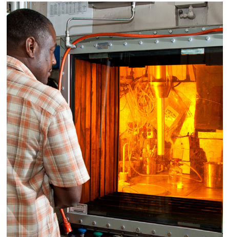
Shielded cells at SRNL
