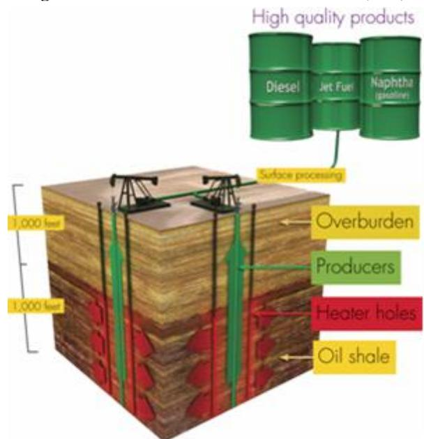
**ICP Nahcolite Test at Site 2:** Shell proposed to conduct an In-situ Conversion Process (ICP) test that would demonstrate the technical feasibility of combining conventional Nahcolite solution mining (using hot water) and extraction methods with the ICP hydrocarbon extraction technology.<sup>36</sup>
