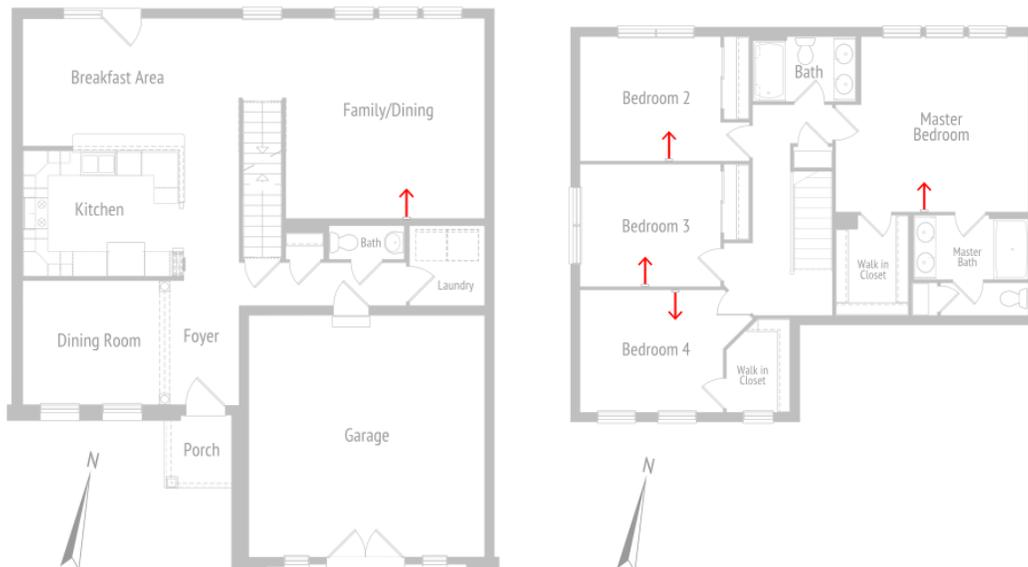
**Figure 3. Low airflow volume ducted distribution to the bedrooms and full volume single point to the main floor: first floor (left) and second floor (right). (The partially open door position shown in the graphic does not represent the door position used in the house during testing.)**
