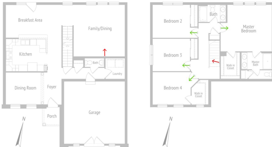
**Figure 4. Over-door powered transfer fans to the bedrooms and full volume single point to the main floor: first floor (left) and second floor (right). (The partially open door position shown in the graphic does not represent the door position used in the house during testing.)**
