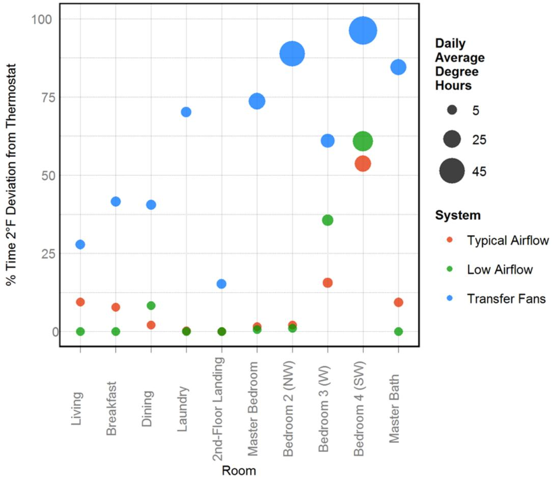
**Figure 10. Percentage of failure time, and extent in degree hours, by room for non-ASHRAE conditions**
