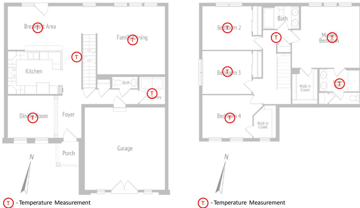
**Figure 8. Sensor locations: first floor (left) and second floor (right). (The partially open door position shown in the graphic does not represent the door position used in the house during testing.)**
