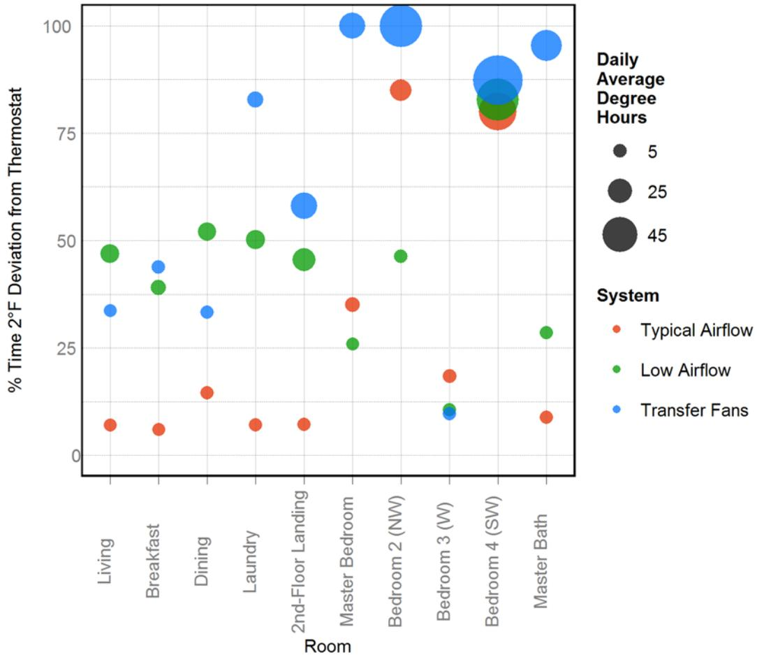
**Figure 9. Percentage of failure time, and extent in degree hours, by room for ASHRAE conditions**
