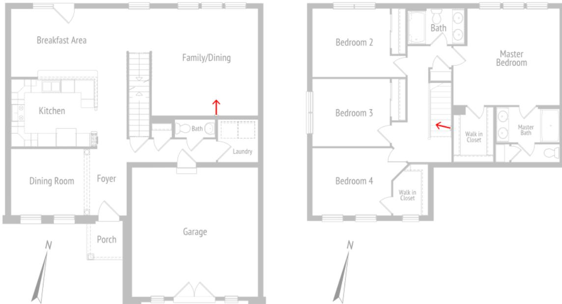
**Figure 7. No ducted distribution to the bedrooms: first floor (left) and second floor (right). (The partially open door position shown in the graphic does not represent the door position used in the house during testing.)**
