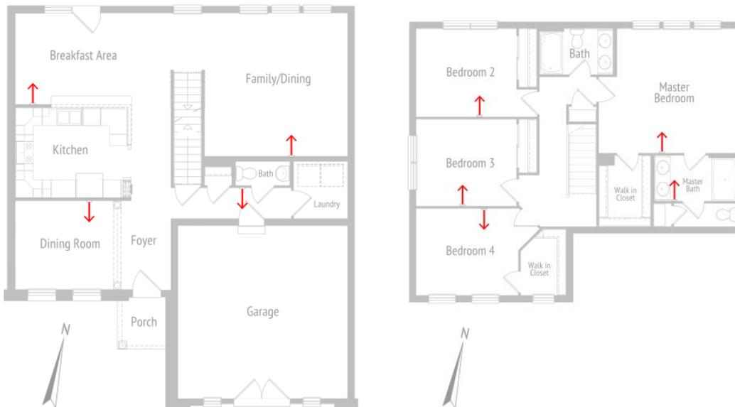
**Figure 2. Typical airflow volume ducted distribution to the bedrooms and all rooms: first floor (left) and second floor (right). (The partially open door position shown in the graphic does not represent the door position used in the house during testing.)**
