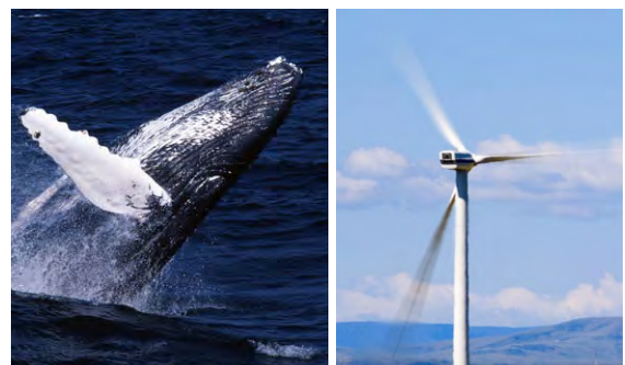
Scientists are mimicking scalloped edges of humpback whales to reduce drag and improve wind turbine design.
