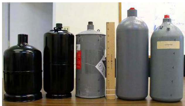
Various flasks used for storing and transporting elemental mercury. Note: All flasks are about 12 inches. See ruler above.
