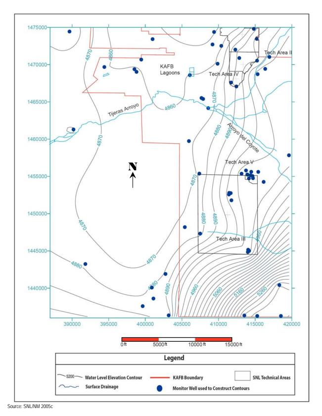
Figure 4.1-1. Elevation Contours of the Regional Groundwater Table
