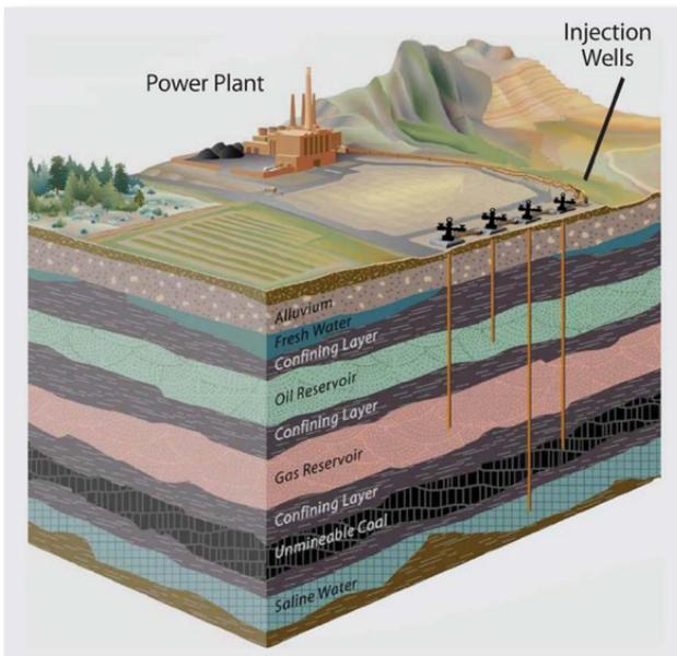
*Carbon capture and storage includes a group of technologies for capturing  $\text{CO}_2$  from power and industrial plants, compressing and transporting it (usually via pipeline), and injecting it for permanent geologic storage in safe underground reservoirs. (Illustration adapted from Energy and Geoscience Institute, University of Utah).*
