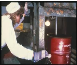
1980 Fernald chemist samples uranium dust collector residue.
